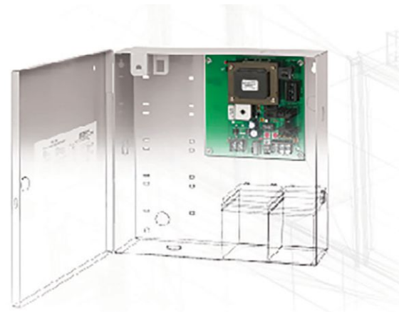
Hybrid power supplies combine the efficiency, or low heat generation, of a switching supply and the rugged inductive load capability of a linear power supply.
