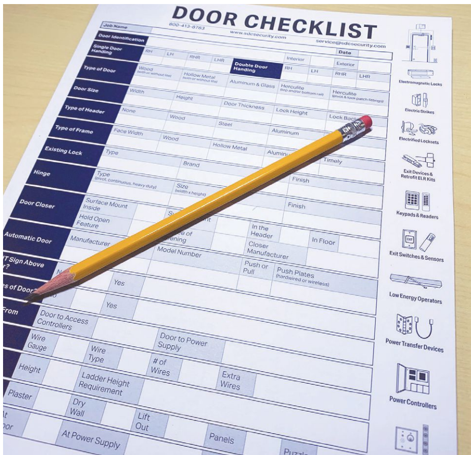
A door checklist can help organize work and make it easier to calculate power loads.
