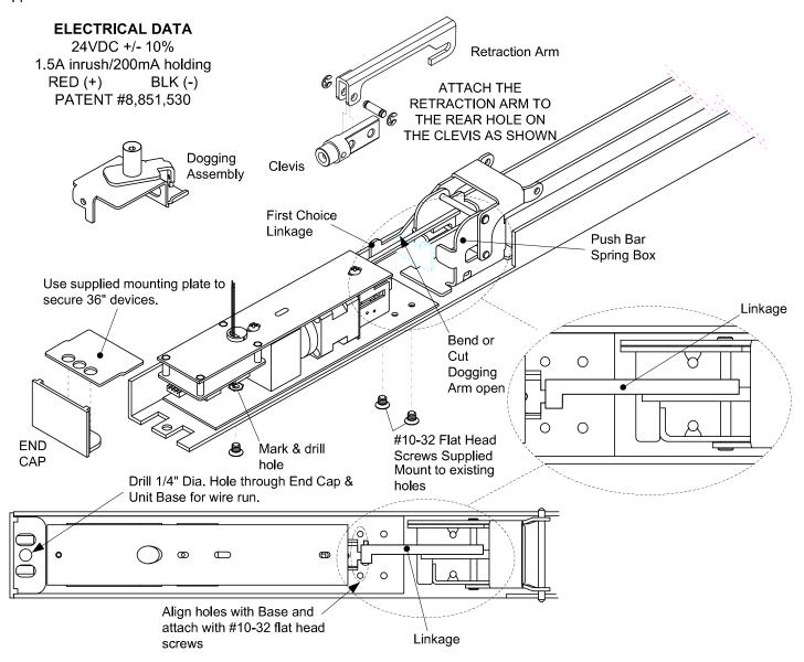
When retrofitting to existing vertical rod devices, adjustment of the rods is required for proper operation of the Electric Latch Retractor. Once the unit is properly installed, energize it so the latch is dogged down, then reconnect the vertical rods to the device and make the proper adjustments.
