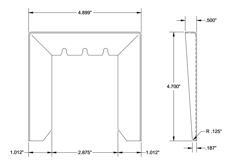
The 480-4SE Mounting box is used between a 4.5" x 4.5" switch and the mounting surface to prevent water and ice infiltration in cold weather
